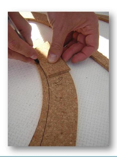
Be sure the trace line is smooth and parallel before cutting. This will ensure the uniformity of the piece. Sand the cut edge and inspect the piece for accuracy
