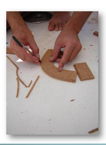
Once cut, you must create the caulking groove. Trace another line 4mm from the edge which will be the cutting line to create the groove.
