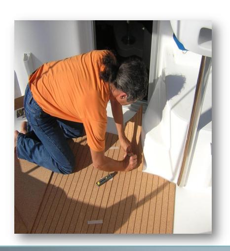
Locate the centre line of your work area and mark it, rough fitting your sheets. At times a pattern might assist in cutting of the sheets for the rough fit.
